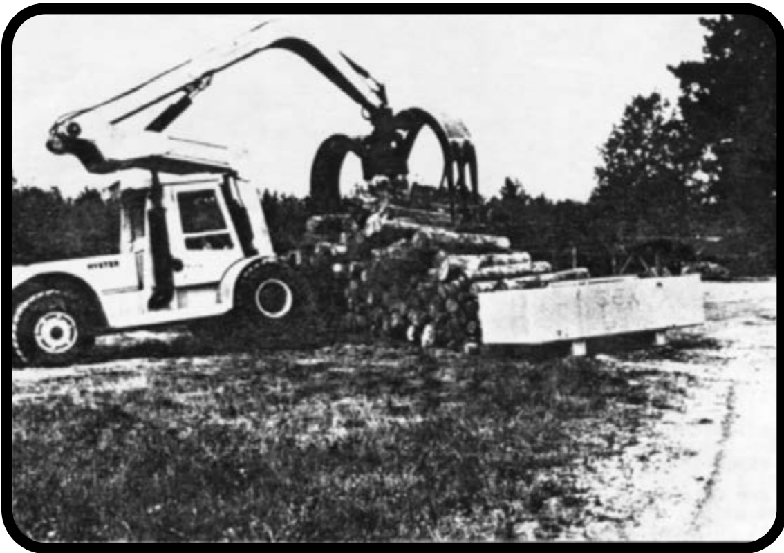
Above shown Hyster being lifted off the ground as it digs into wood stack.
